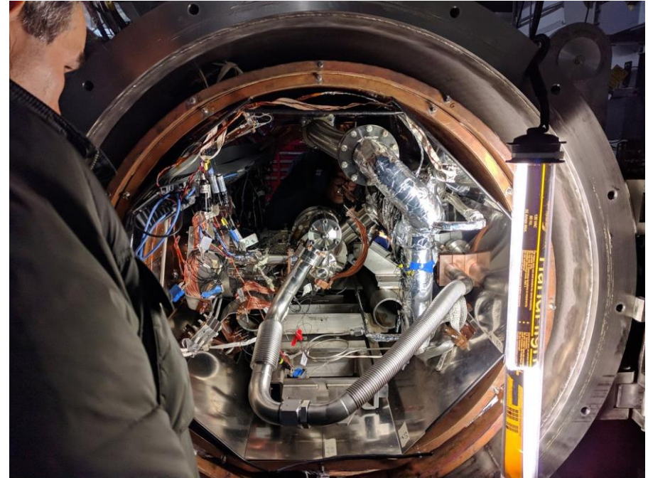
3.9 GHz LCLS-II Dressed Cavity installed at the Horizontal Test Cryostat at FNAL
